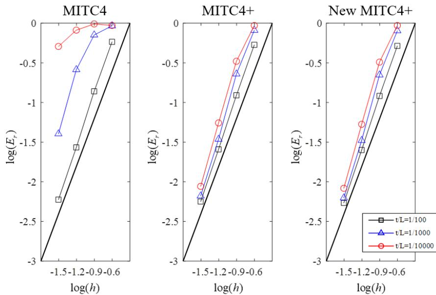
Fig. 6 Convergence curves for the free cylindrical shell problem with distorted meshes
