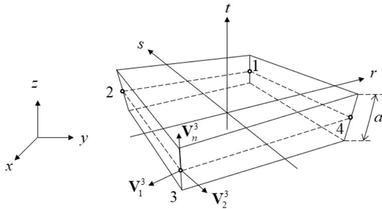
**Fig. 1** A 4-node quadrilateral shell finite element.
