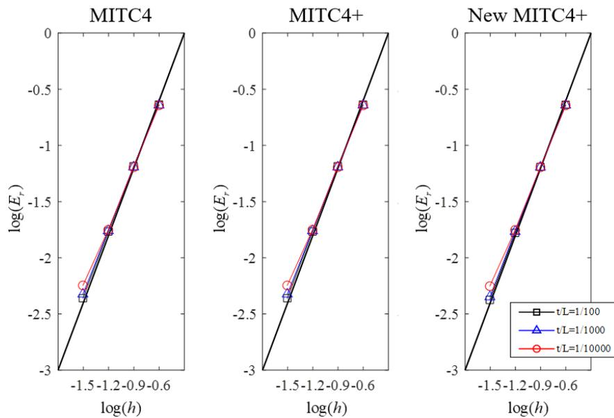
**Fig. 5** Convergence curves for the free cylindrical shell problem with regular meshes
