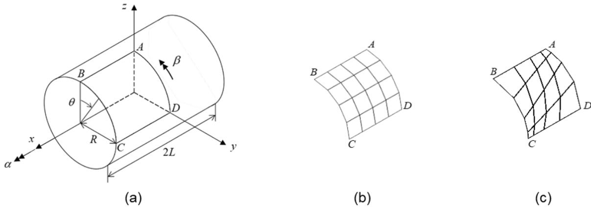
**Fig. 4** (a) Cylindrical shell problem ( $L = R = 1$ ,  $E = 2.0 \times 10^5$ , and  $\nu = 1/3$ ). (b) Regular mesh when  $N = 4$ . (c) Distorted mesh when  $N = 4$ .
